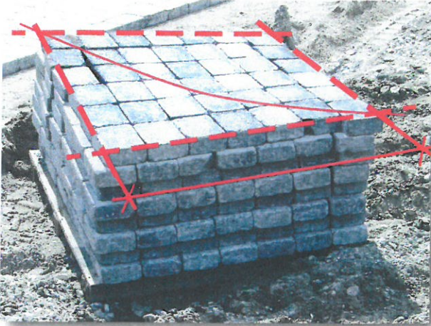
Site-problem: Uneven packs: TWIST stone layers
