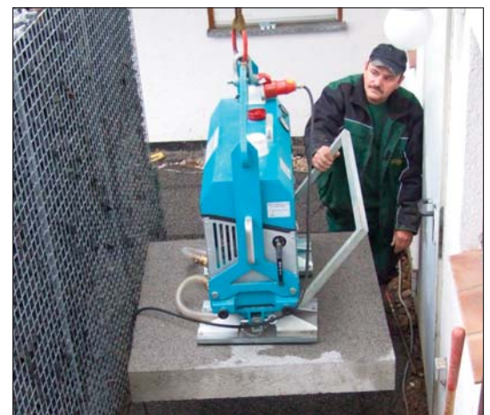
Kappa Levator with electric motor, carrying capacity 800 kg.
